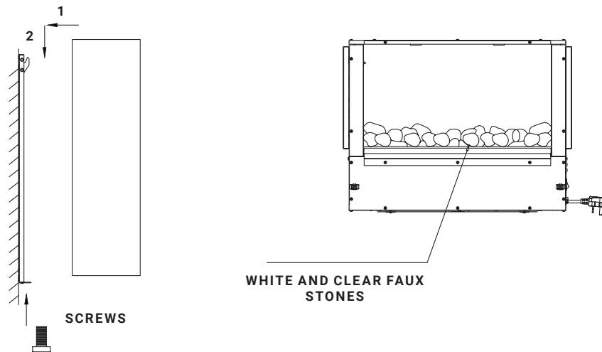
**2.4** Hang the glass pane to the fire chamber, press the front of the glass and attach it to the surface of the fire chamber using 2 screws (M4 x 8).
