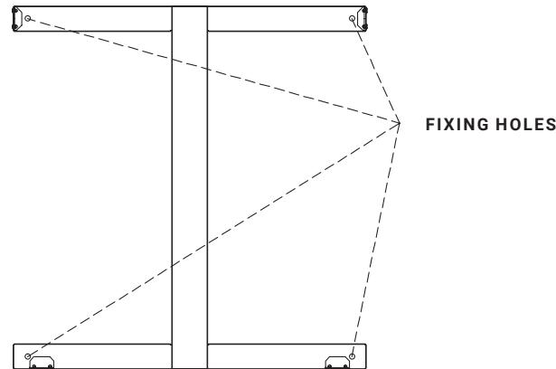
**2.2** Drill the four marked holes using an 8 mm drill. Tap the plastic dowels into the holes. If the wall is made from solid wood, it is not necessary to drill the holes or use the plastic dowels. Next, attach the wall bracket using 4 screw (ST5x40).
