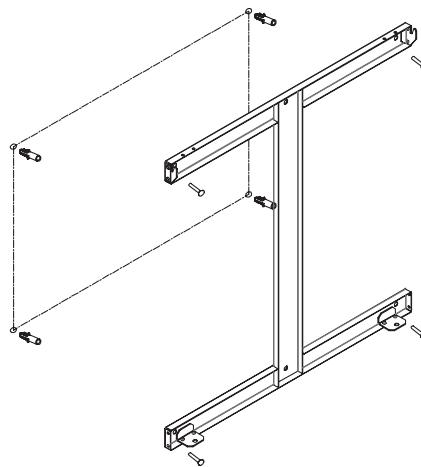
**2.3** Attach the fire chamber to the bracket and secure it using 2 screws (M5 x 10) on the underside of the fire chamber. Arrange the decorative materials in the EF159P along the bottom of the fire bed as desired.
