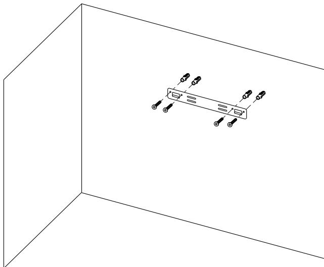
Lift the appliance up and attach to the wall bracket, mark the hole position of the two bottom fixing brackets, take the appliance down, drill holes on the marks and then insert wall plugs into it.
