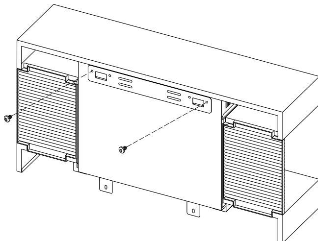
Place the wall mounted bracket in the desired position ensuring that the bracket is level. Mark and drill the fixing points, tap wall plugs into the holes and secure the bracket to the wall with 4x ST5\*40 Screws.
