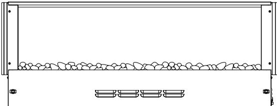
**2.5** Mount the front glass sheet and secure it using two ST4X10 screws.
