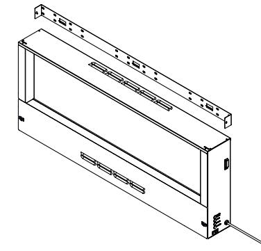
**2.2** Remove the bracket and drill the 6 holes Ø8 into the wall. Tap the plastic dowels into the holes. If the wall is made from solid wood, it is not necessary to drill the holes or to use the plastic dowels. Next, attach the wall bracket using 4 screws (ST5 x 40).
